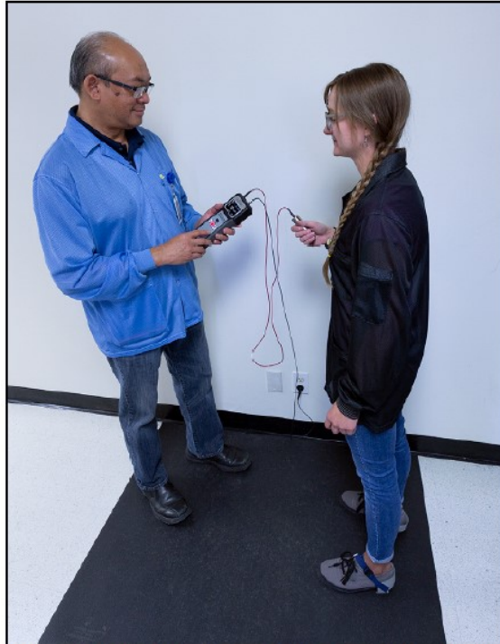
Figure 10. Using the Desco 19295 Handheld Electrode to measure the Resistance-to-Ground (Rtg) of an operator wearing foot grounders
